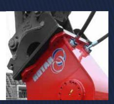
The position of the hydraulic cylinder is designed at an optimum angle. This angle ensures a constant, powerful penetration during the complete stroke
